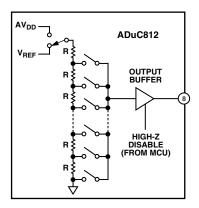
Figure 18. Resistor String DAC Functional Equivalent
